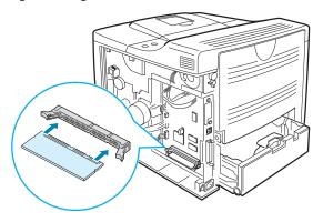
4 Replace the control board cover and tighten the two screws.
